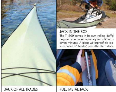
The side jacks hook the hull right or left, giving the bow a kinked-up look. This may be useful for tracking in wind and waves with no rudder or skeg.
